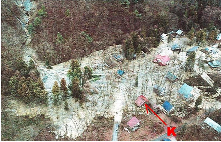
Debris flow from a small valley above reached to the Hakuba branch (K mark). Photo by the Hakuba Village.
